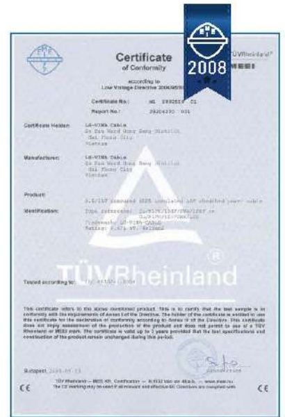
Type of cable : 0.6/1 kV Cu/XLPE/LSHF/SWA/LSHF 4x16mm² Test Standard: IEC 60502-1:2004
