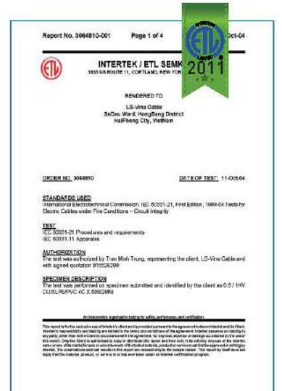
Type of cable : 0.6/1kV Cu/XLPE/PVC 4x50mm² Test Standard: IEC 60331-21; IEC 60331-11
